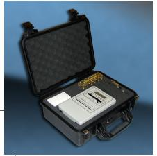
The 311XL and 311TCXL are portable, intrinsically safe trace oxygen analyzers which can be operated without an external power source, providing analysis in decade steps ranging from 0-2 to 0-10,000 ppm full scale plus a special
