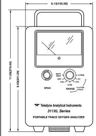
Measurements are given in inches and millimeters. The instrument is 5 - 5/8" (142.8mm) deep.
